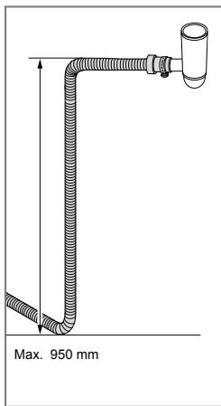
The drainage hose can also be connected to a connection nipple on the sink unit's water trap. The connection nipple must have an internal diameter of at least 14 mm.
