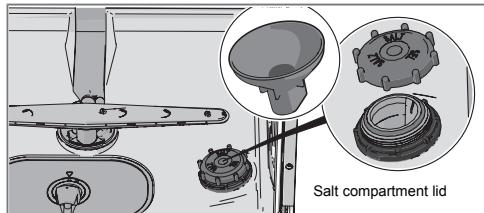
When the salt runs out, unscrew the cap and fill the container with salt. Water is only needed the first time! Wipe clean and tighten. Run a program to ensure that any salt in the dishwasher is rinsed away.
